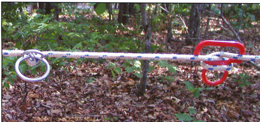
The Clemson Easy Tie (left) and the Knot Eliminator (right) are both easy to pack and use a minimum amount of line length.
