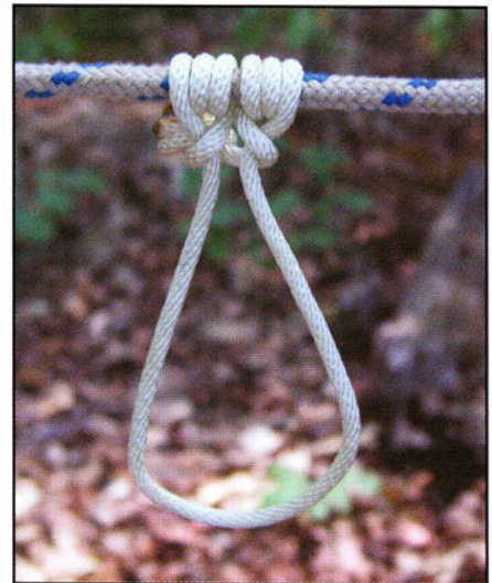
The Prussik knot is placed on the line after it has been secured and tightened.
